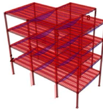
Figure 18: Structural: Structural analysis results (bending moment, shear force and deflected shape)
