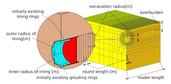
Fig. 4: Geometrical parameters of the FE simulation model.
