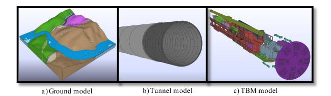
Fig. 2: Components of the proposed IFC tunnel product model: (a) the ground data model (GDM), (b) the tunnel model (TM), (c) the tunnel boring machine model (TBM).
