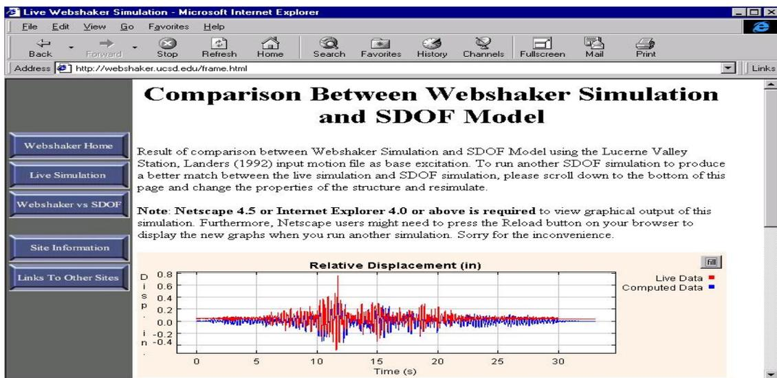
Figure 4. Sample Comparison between first floor recorded and computed response.
