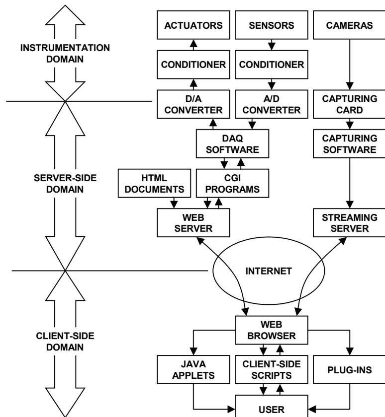
Fig. 1. Layout of Internet monitoring and control system.
