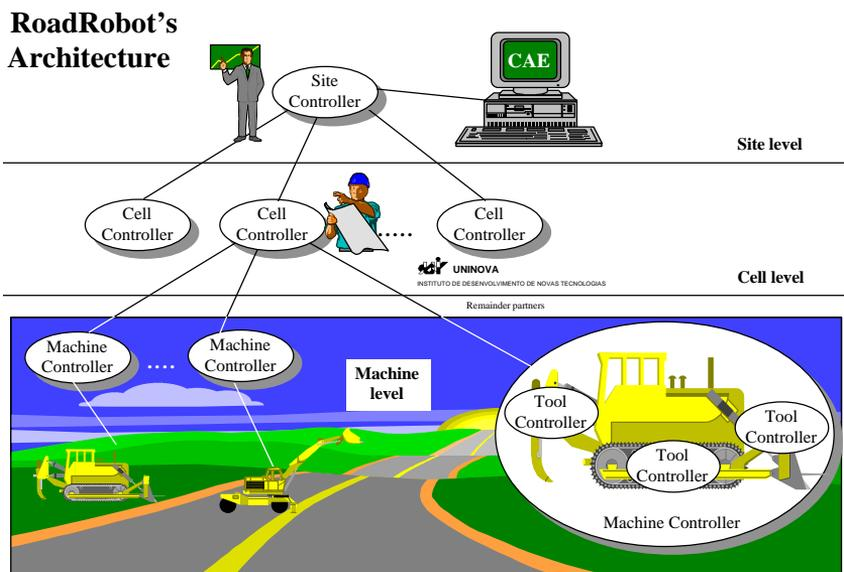
Figure 2. Architecture of RoadRobot project - Logical levels
