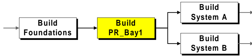
Figure 2. Partial view of activity network used to plan and manage the construction of the Deethanizer Unit.
