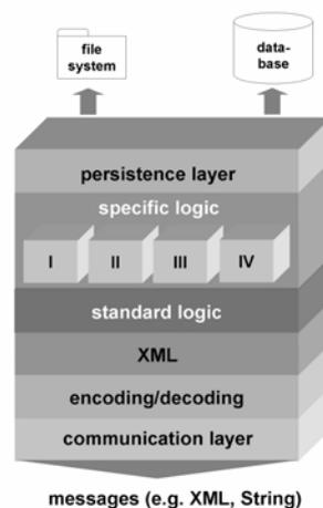
Figure 3 Conceptual design of the agent architecture
