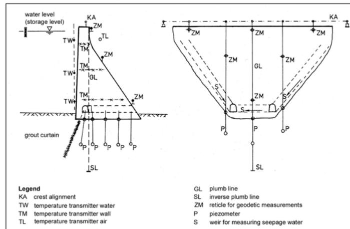
**Figure 1** Example for the configuration of measuring devices [1]
