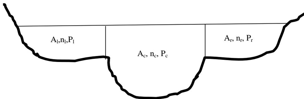
Figure 2: Division of the Flooded Natural Cross Section into Discrete Elements
