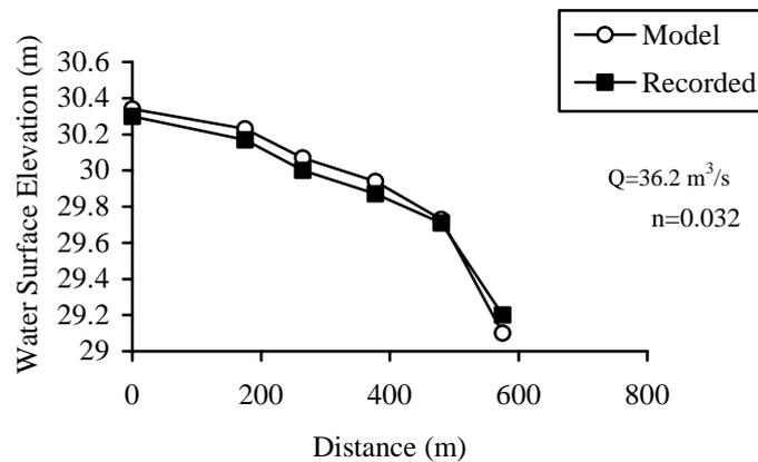
Figure 3: Measured and Predicted Water Surface Elevation of the Linggi River
