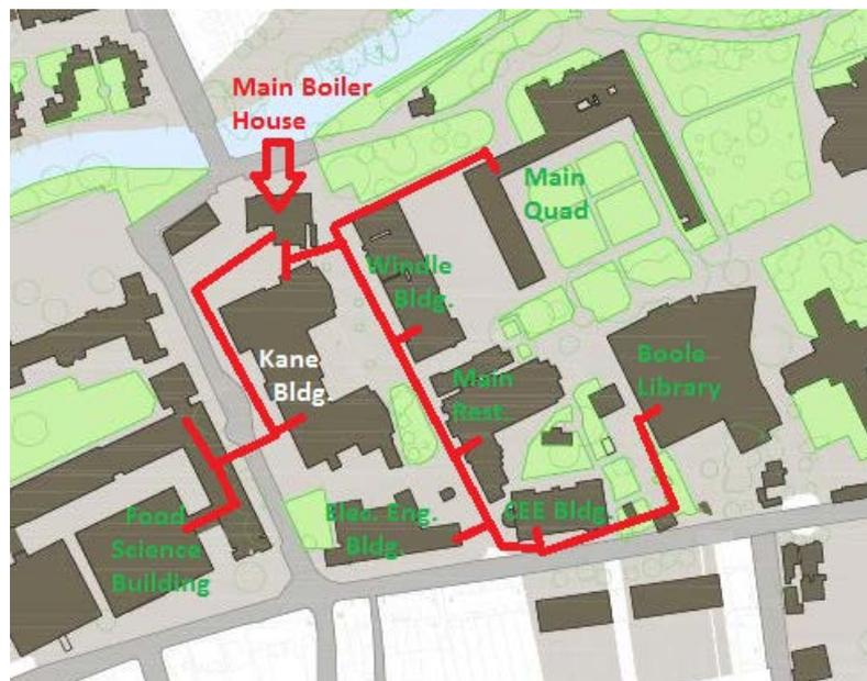
Figure 3: Campus Heating Energy Connections to Main Boiler House
