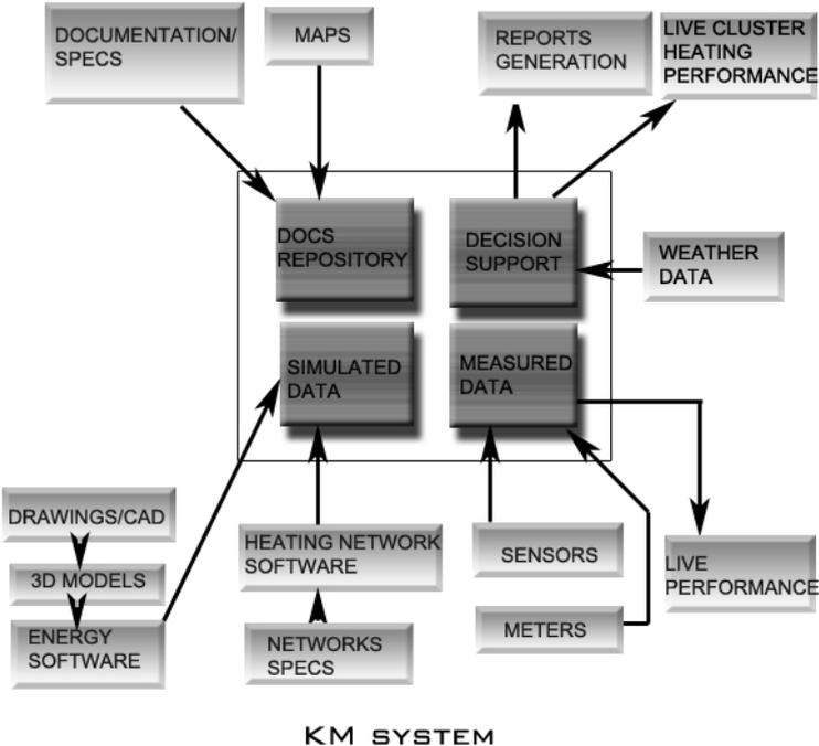
Figure 2: Knowledge Management system for campus heating system management.
