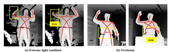
Figure 1. Limitations of Kinect
