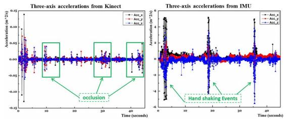
Figure 4. Three-axis accelerations captured in preliminary experiment
