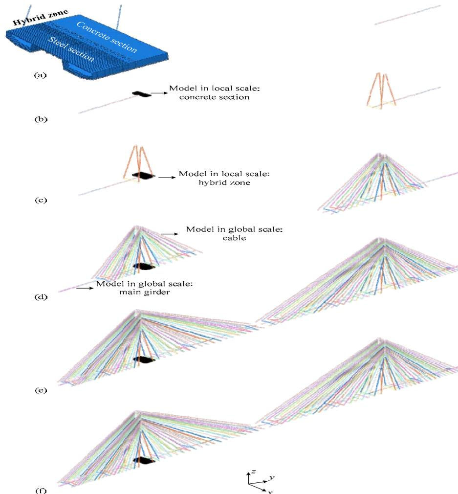
**Figure 4. FE models. (a) traditional local-elaborate model; (b) 4D Multi-scale model, *P-I*: concrete section up; (c) 4D Multi-scale model, *P-II*: steel section up; (d) 4D Multi-scale model, *P-III*: 9<sup>th</sup> cable on; (e) 4D Multi-scale model, *P-IV*: last cable on; (f) 4D Multi-scale model, *P-V* and *P-VI*: bridge complete and on service.**
