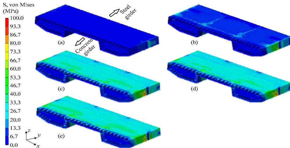
**Figure 6. Distribution of von Mises stress of steel section in hybrid zone using 4D multi-scale modeling method. (a) *P-II*: steel section up; (b) *P-III*: 9<sup>th</sup> cable on; (c) *P-IV*: last cable on; (d) *P-V*: bridge complete; (e) *P-VI*: bridge on service.**
