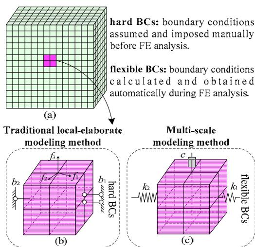
**Figure 2. Multi-scale modeling method. (a) real structure; (b) traditional local-elaborate model; (c) multi-scale model.**
