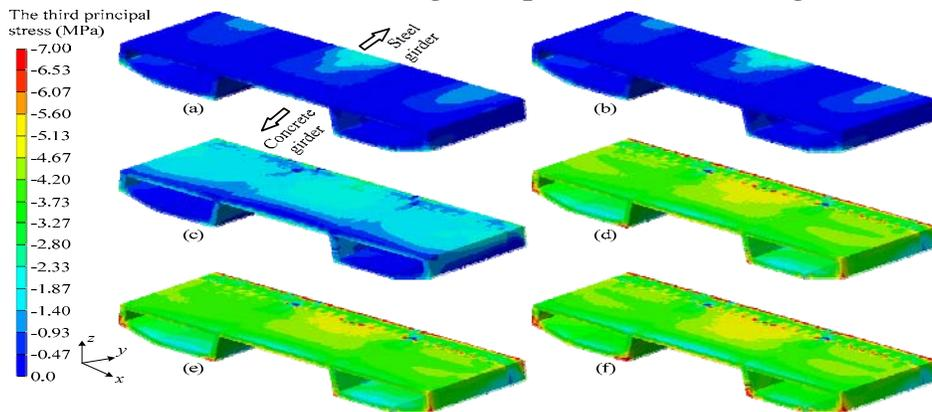
**Figure 7. Distribution of the third principal stress of concrete section in hybrid zone using 4D multi-scale modeling method. (a) *P-I*: concrete section up; (b) *P-II*: steel section up; (c) *P-III*: 9<sup>th</sup> cable on; (d) *P-IV*: last cable on; (e) *P-V*: bridge complete; (f) *P-VI*: bridge on service.**
