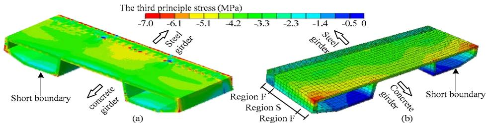
**Figure 5. Distribution of the third principal stress of concrete section in hybrid zone at *P-IV*. (a) 4D Multi-scale model; (b) traditional local-elaborate model.**
