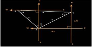
Figure 2. Frame 1: Symbolic and graphical representations of the math concepts used to calculate the coordinates of a point of interest C from two points of known coordinates A and B
