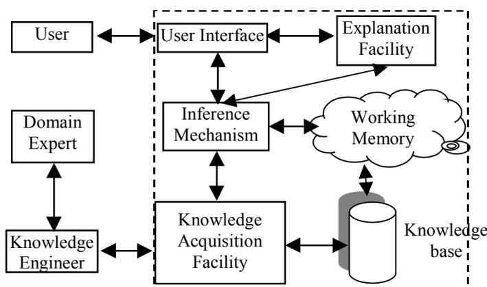
Fig. 3 Illustration of a KBES
