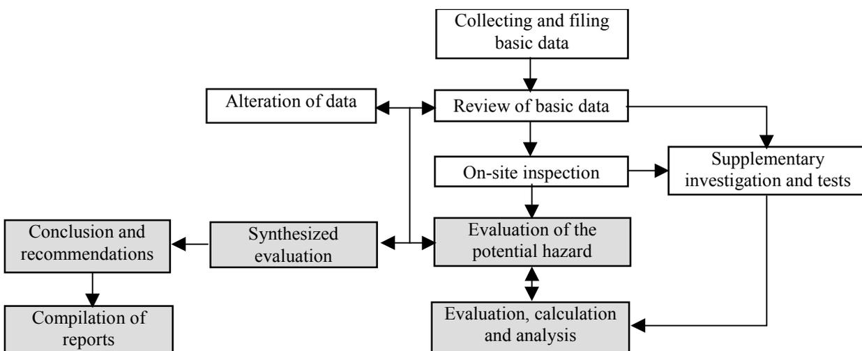
Fig. 1 Flow chart for conventional dam safety inspection in Taiwan
