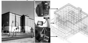
Figure 1: Current building surveying process, Left: Building Surveying. Middle: Laser Distance meter, Total Station and Photogrammetry. Right: Geometry Model – CAD
