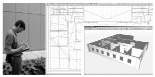
Figure 11: Plan-oriented and 3D-views of a geometry model using the tools "OpenGLviewer" and "PlanarViewer", showing an example of a manually measured survey of a building
