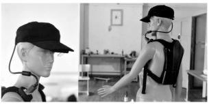
Figure 18: design study - cable route model from connector to HMD [15] and model of backpack-like wearable computer [14], [16], [17], [18]
