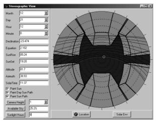
Figure 8: Solar path depending on the time of the day.
