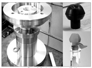
Figure 2. Synthetic cork for gasified beverages.
