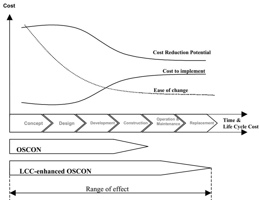
**Fig. 2: Project life cycle phases and OSCON application**
