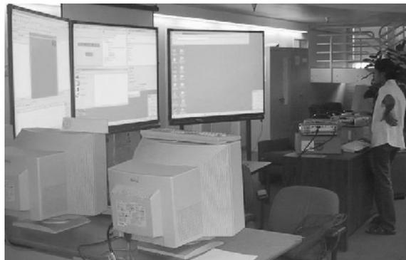
*Fig. 2: The CIFE iRoom. There are three, front-projected SMART Boards with touch panels, plus a wireless keyboard and mouse.*
