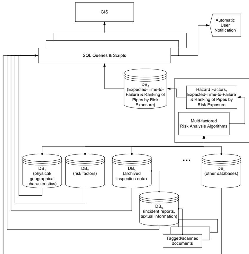
Figure 1: GIS-based management system for water distribution networks (database structure)
