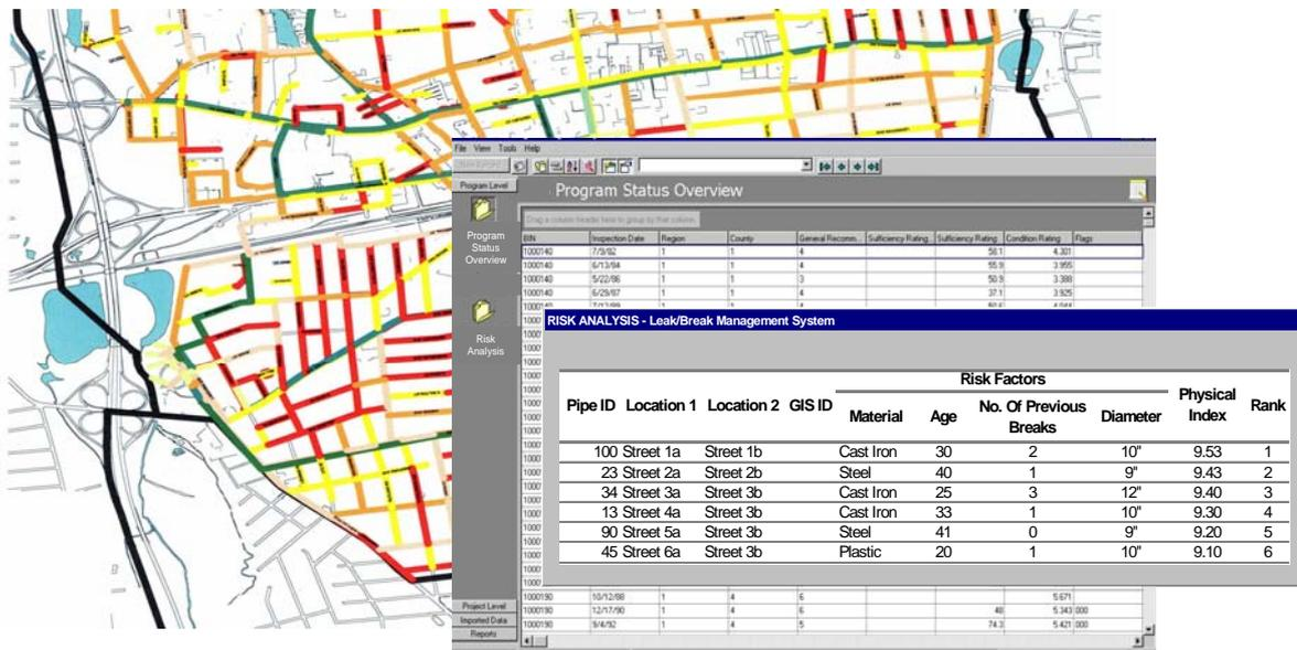
Figure 1: GIS-based management system for water distribution networks (graphical interface)
