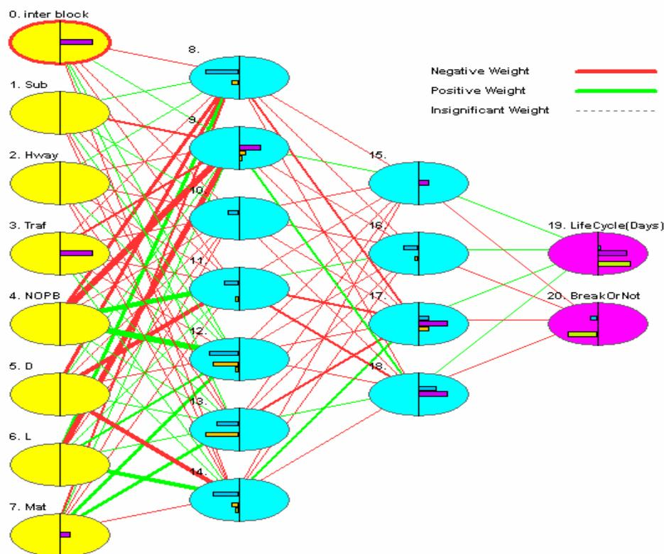
Figure 3: Artificial neural network (ANN) model of the risk factors for failure
