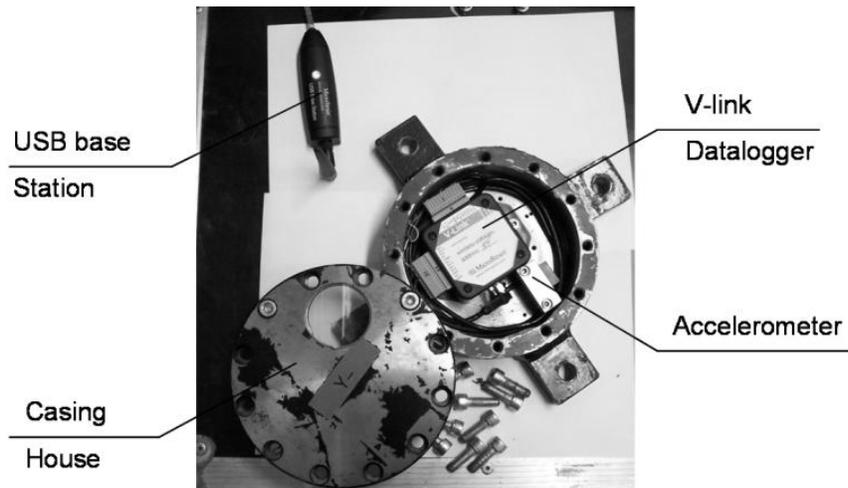
Figure 2: Device used to acquire deceleration history of rock impact
