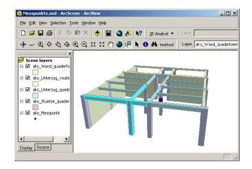
Figure 4: 3D representaion of building model data in a GIS
