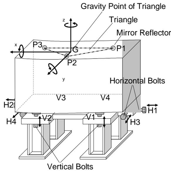
Figure 5: Gravity Point of Triangle and 3 rotational axes on Electromagnet
