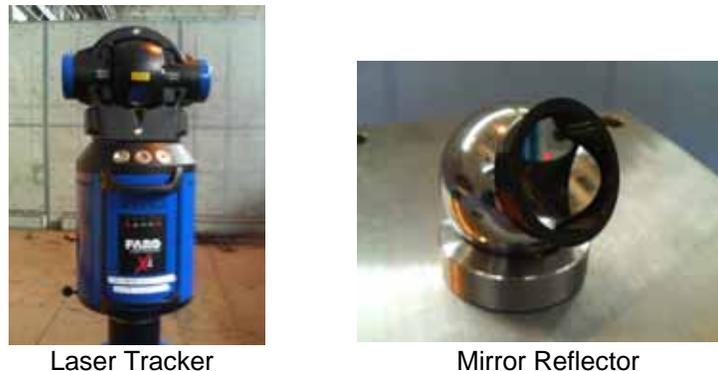
Figure 4: Laser Tracker and Mirror Reflector
