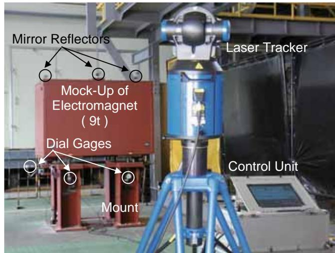
Figure 2: Alignment System
