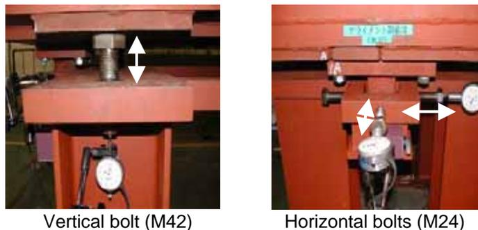
Figure 3: Position Adjustment Bolts and Dial Gages attached to them
