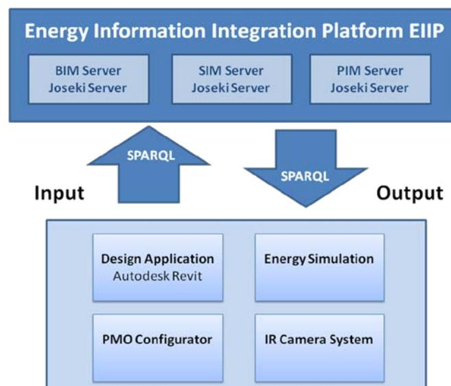
Figure 6: Energy Information Integration Platform (EIIP) data flow.
