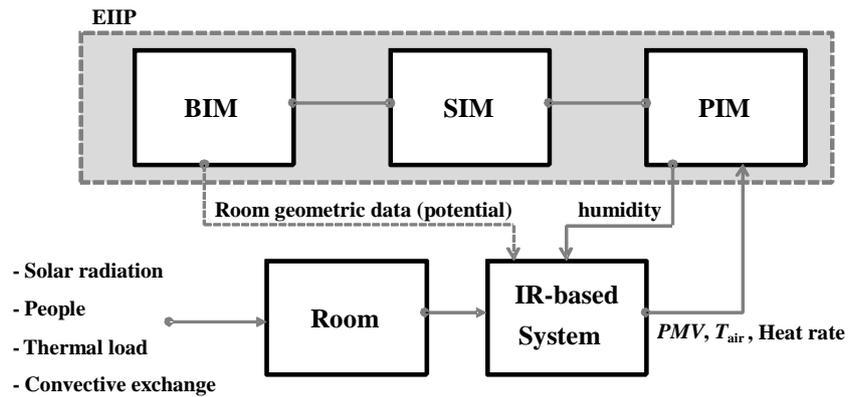
Figure 1: IR-based system data flow integrated with the EIIP architecture.
