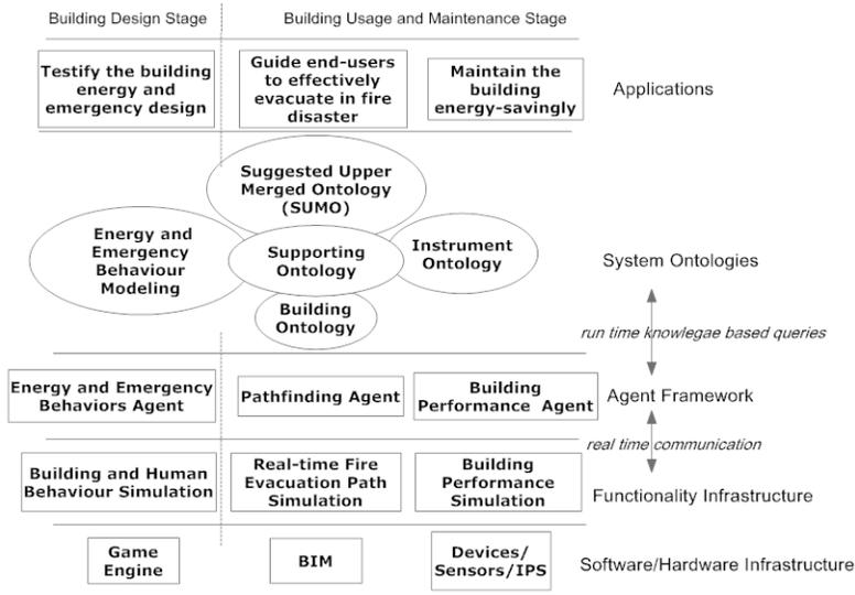
Figure 5: Four layered framework of virtual building system (Dibley et al., 2012a)
