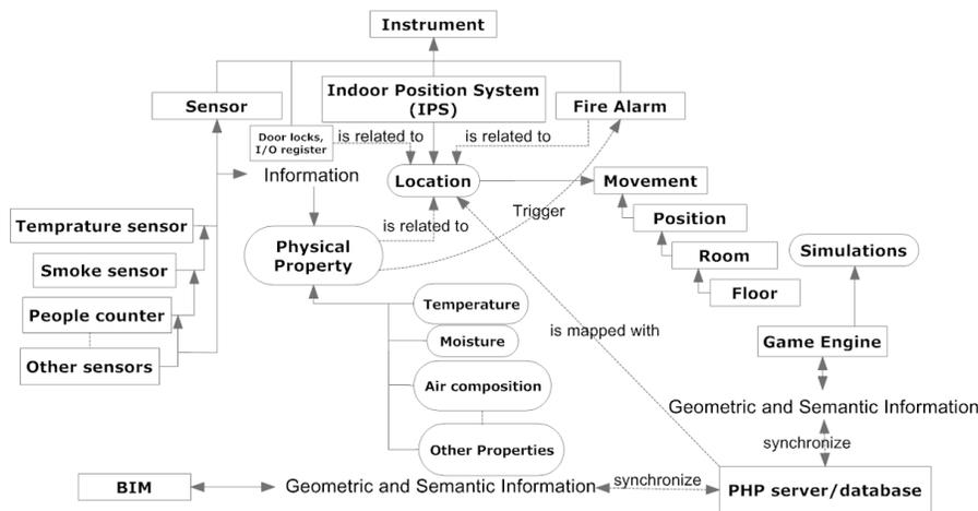
Figure 6: Instrument ontology related to key object factors during a fire evacuation (Mion et al., 2008)
