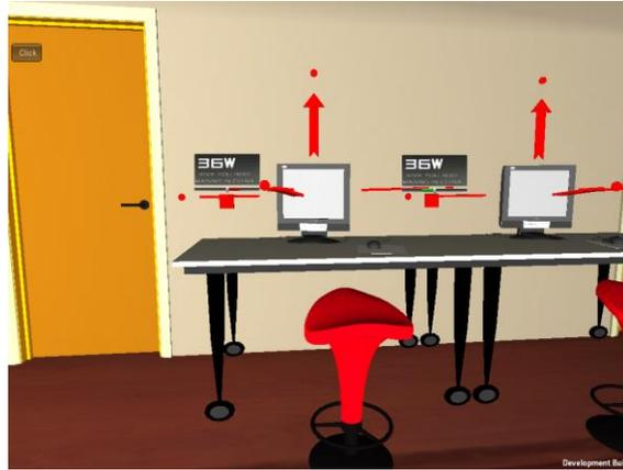
Figure 8: Monitoring air flows using arrow graph and power consuming with bar graph in 3D
