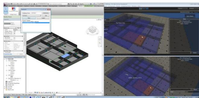
Figure 4: Automatic data transmitting between Revit and Game Engine for real-time fire evacuation path simulation
