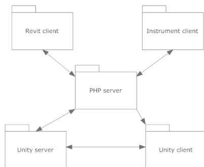
Figure 3: The package diagram for automatic data transmitting
