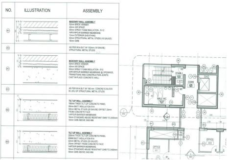
Figure 1: Style of designating and defining wall types and applying it to an actual design
