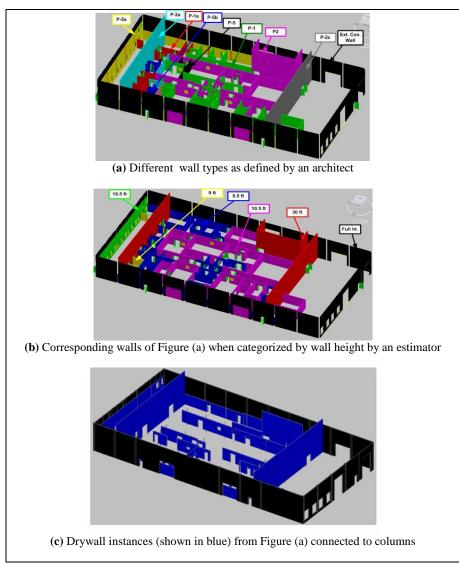
Figure 6: Grouping of walls using different criteria
