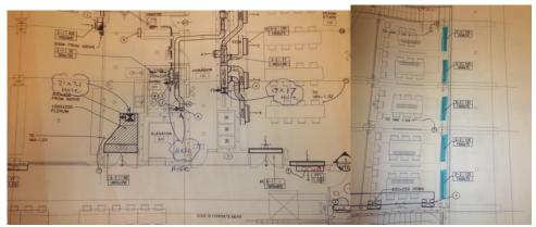
Figure 7: Hand marking of (a) the size of duct penetrations on a portion of a slab and (b) the openings in structural walls
