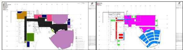
Figure 4: Colour-marking of different (a) floor finishes in the floor plan, and (b) ceiling types and finishes in the reflected ceiling plan
