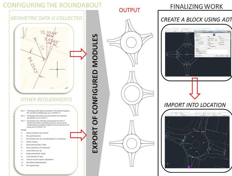
Figure 3: Use of configurator on the internal website and finalizing work.
