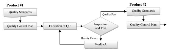
Figure 2. Quality Control Process Flowchart.
