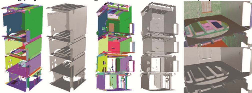
Figure 6. Segmentation and NURBS fitting of a scene from multiple laser scans.
