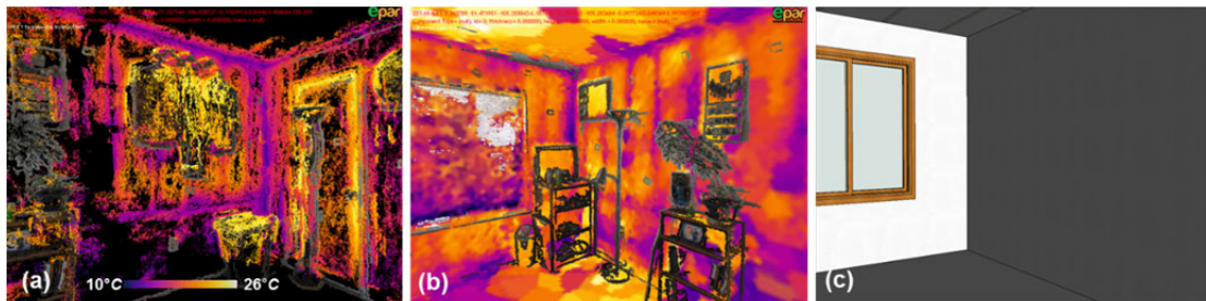
Figure 2. (a) 3D thermal point cloud and (b) mesh models jointly visualized with the building geometry, and (c) BIM of the same building environments.
