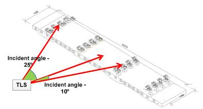
Figure 4. Effect of incident angle on dimensional estimations
