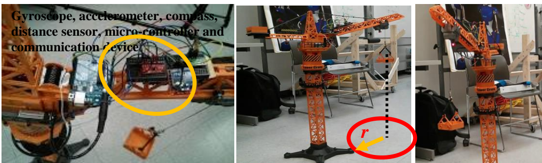
Figure 3. Dangerous zone under the load of swinging crane
