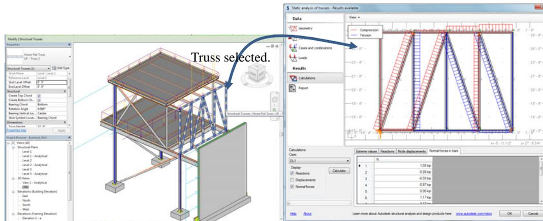
Figure 5. Truss analysis tool.
