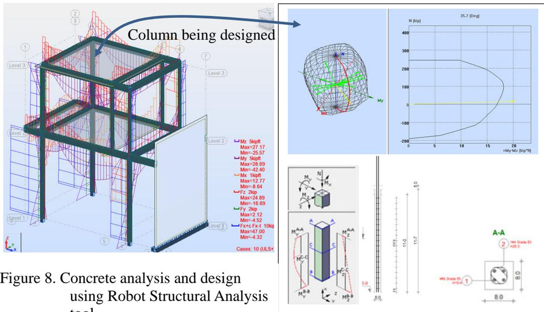
Figure 8. Concrete analysis and design using Robot Structural Analysis tool.
