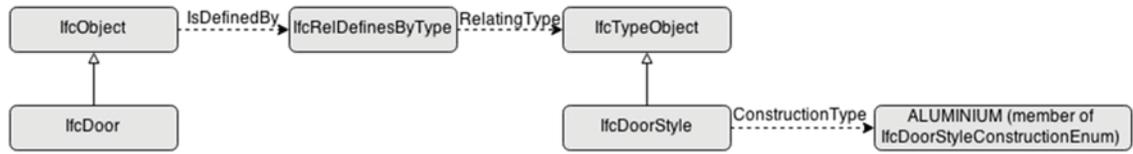
Figure 1 Path between the entities IfcDoor and ALUMINIUM
