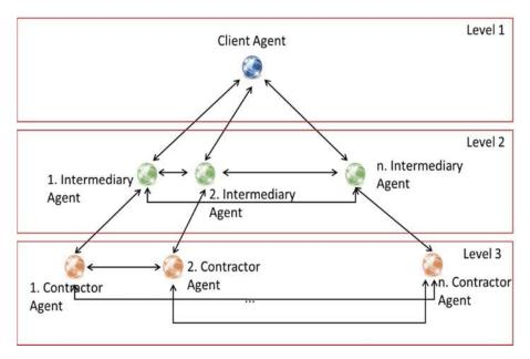
Figure 2 The Agent Interaction Levels of the Multi-Agent System based Contractor Prequalification and Selection Model
