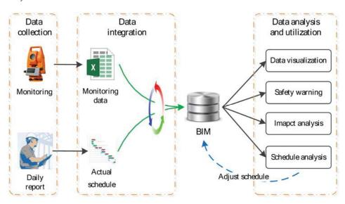
Figure 3 Workflow for settlement monitoring and impact management
