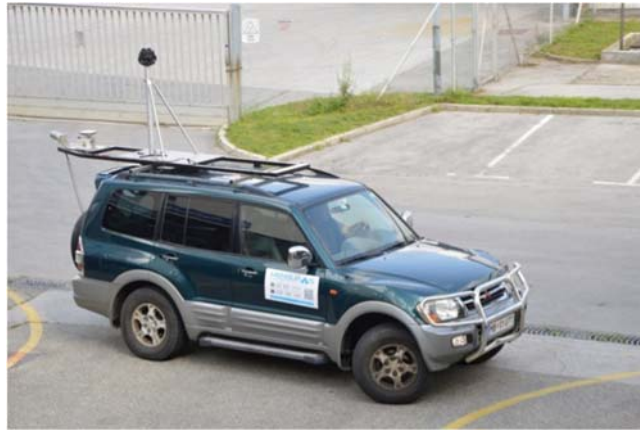
Figure 9. A car with mounted LiDAR device (courtesy of Mensuras d.o.o.)
