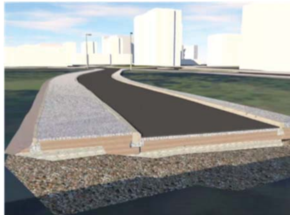
Figure 8. Cross-section cut of the new road segment
