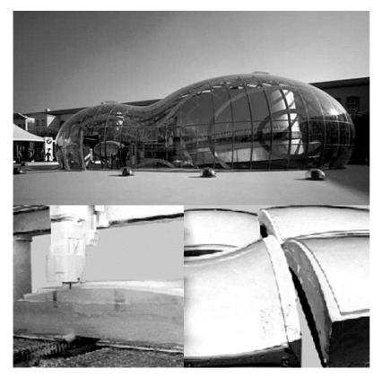
Fig 6. Milling of molds for acrylic glass panels in Bernard Franken's BMW pavilion.
