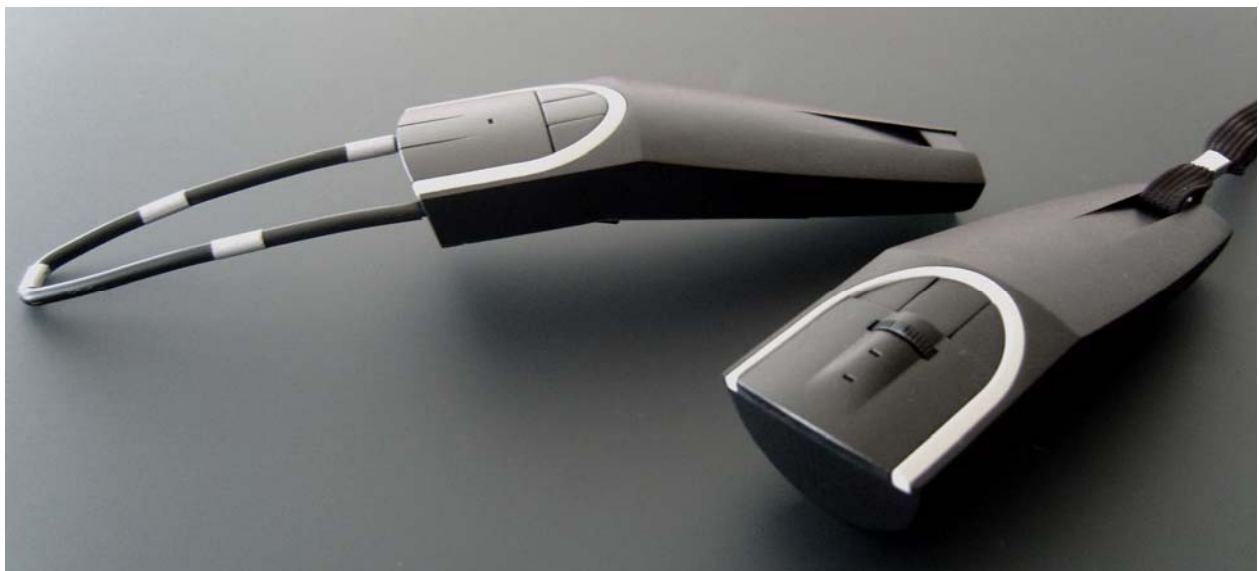
FIG. 9: Input device - 3D interaction device (left), recording device (right)
