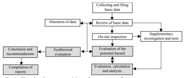
Fig. 1 Flow chart for conventional dam safety inspection in Taiwan
