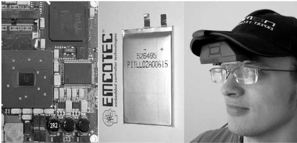
Figure 15: Using commercially available components, Left: PC-mainboard (3.7x4.5" , Pentium® M 1.6 GHz, 512 MB), Middle: Rechargeable batteries from model building technology, Right: Retinal display system [15]
