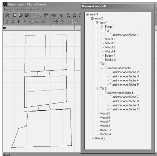
Figure 10: sketch-oriented view – Recording of the spatial structure and essential room-descriptive elements
