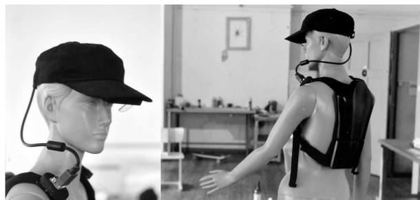
Figure 18: design study - cable route model from connector to HMD [15] and model of backpack-like wearable computer [14], [16], [17], [18]
