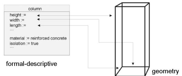
Figure 5: Geometric and semantic structure
