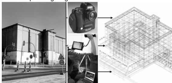
Figure 1: Current building surveying process, Left: Building Surveying. Middle: Laser Distance meter, Total Station and Photogrammetry. Right: Geometry Model – CAD
