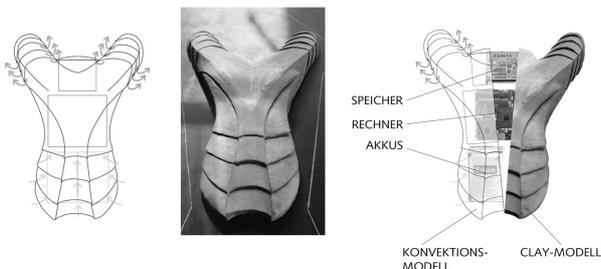
Figure 17: wearable-chassis model made of sheds to provide high flexibility and ventilation [14], [16], [17], [18]
