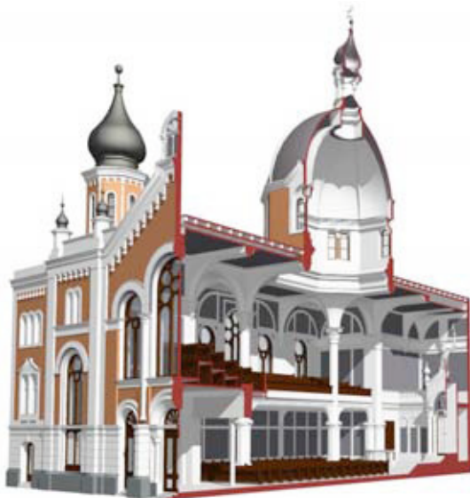
Fig. 13. Demonstration of a “non-destructive cut” in the 3D-Model of the Synagogue in Humboldtgasse.
