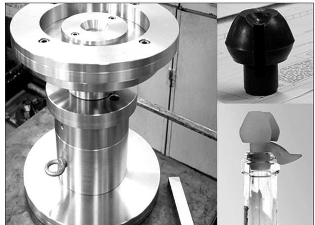
Figure 2. Synthetic cork for gasified beverages.
