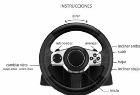
Figure 2. Interaction device and control schema
