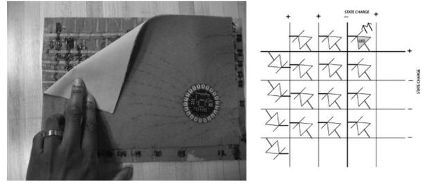
Fig. 4. Conductive Thread Traces on Textile Connecting to Charlieplex Weave (left), Charlieplex Diagram (right)
