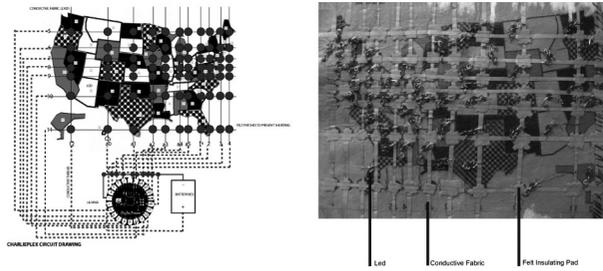
Fig. 3. Circuit Weave (right), Back of Textile (left)
