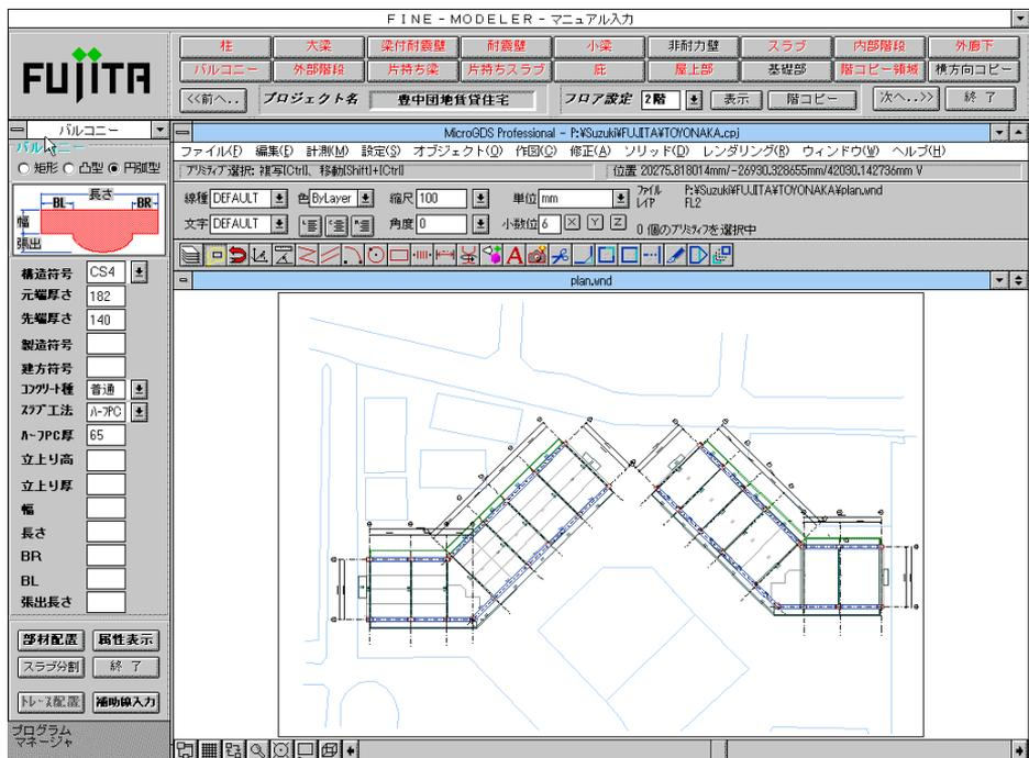
Figure 3: An example of Slab members input by FINE-MODELER
