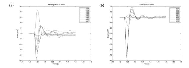
Figure 8: (a) Bending strains for the culvert at profile P2 during impact and (b) Axial strains for the culvert at profile P2 during impact
