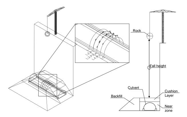
Figure 1: Illustration of experimental setup
