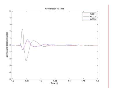
Figure 7: Accelerations for the culvert at profile S2 during impact
