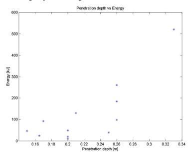
Figure 5: Pentration depth vs Energy for rockfall tests with rock masses of 200, 500, 938 and 2650 kg. Fall heights varying from 5, 10 and 20m
