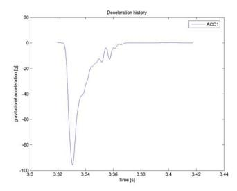
Figure 6: Typical deceleration history of low-energy rockfall impact
