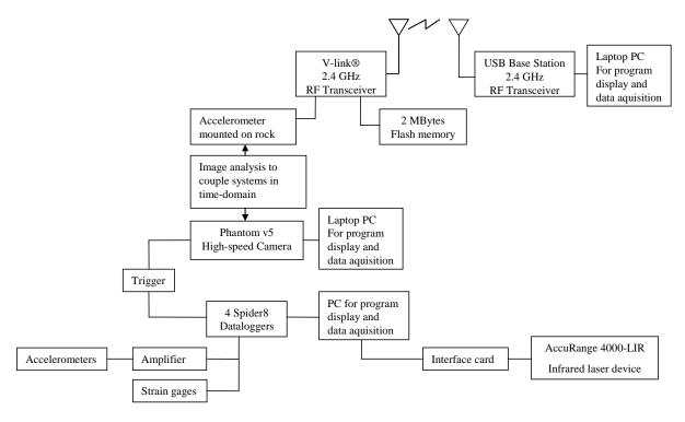
Figure 4: Schematic layout of data acquisition system
