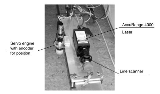
Figure 3: Laser device mounted on wagon. Used inside the tunnel to obtain deformation of culvert
