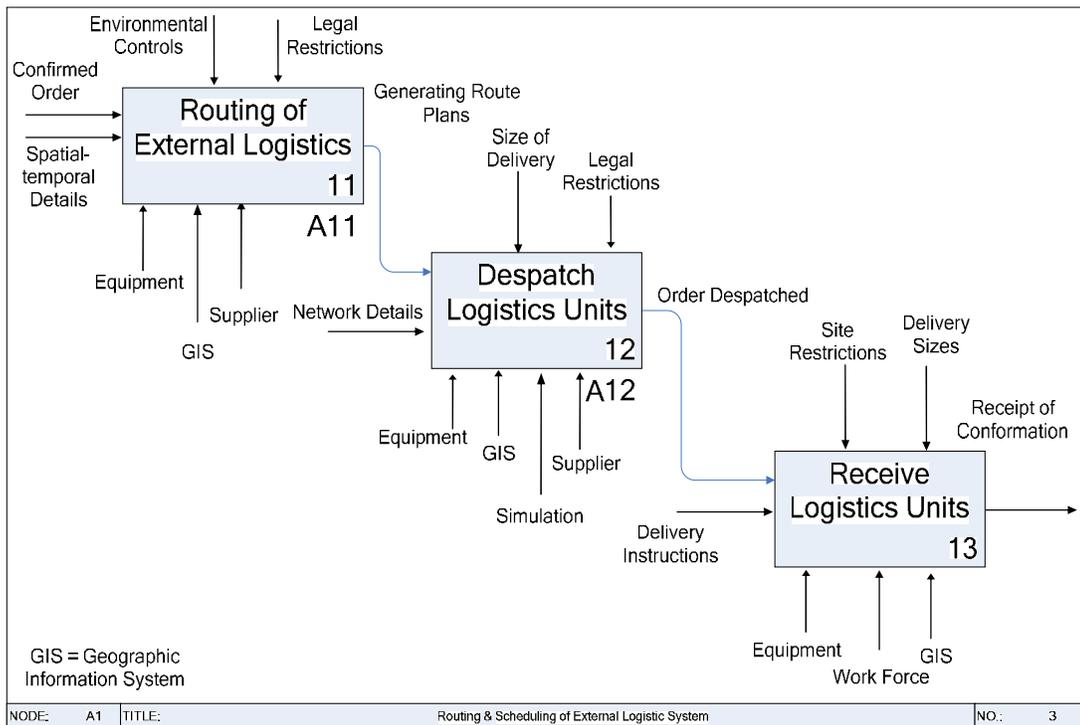
Figure 3: IDEF0 for Routing & Scheduling of External Logistics System
