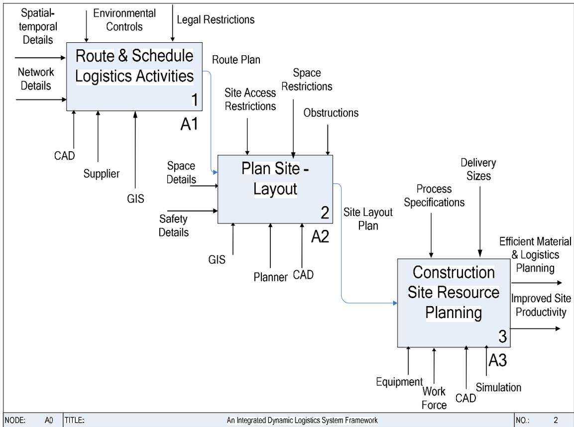
Figure 2: IDEF0 for an Integrated Dynamic Logistics Framework
