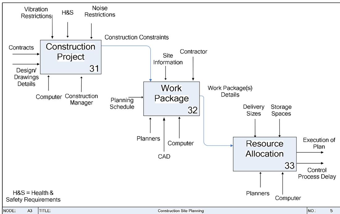
Figure 5: IDEF0 for Construction Site Resource Planning
