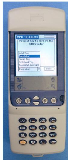
Figure 3 RFID Hand-held reader ([www.rf-id.com](http://www.rf-id.com))
