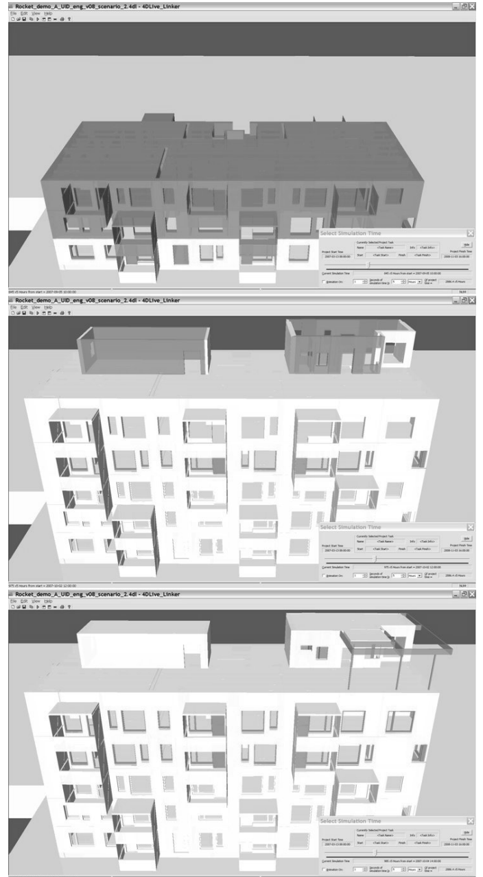
Figure 6. Residential housing simulation in on-site bathrooms scenario, dark elements are under construction.
