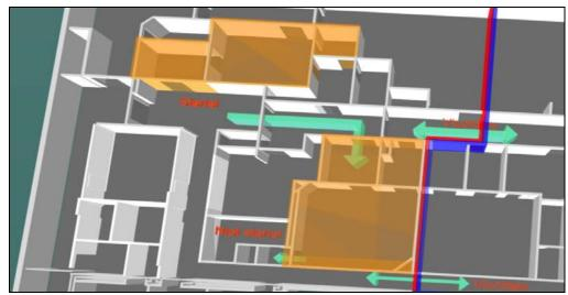
Figure 2: A 4D model generated with the method. Arrows visualize pathways for doctors, surfaces are used to signify areas of medical activity. Additional, elements show dust barriers. Finally, annotations provide additional information.
