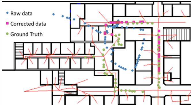
Figure 8. Inertial positioning data correction using weighted topology map-matching algorithm
